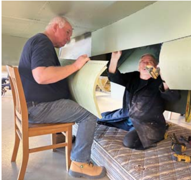
Greenwood Military Aviation Museum volunteers Garry Brown, left, and Dan Daigle fit fabricated replacement bomb bay doors to the underside of the GMAM's restoration Bristol Bolingbroke – its first new bomb bay doors since they were torn off in 1943.
