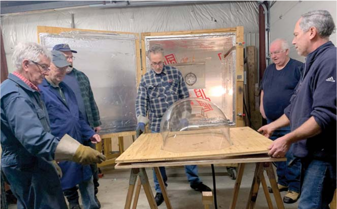
After crafting 16 restoration Lancaster aircraft Plexiglas pieces, volunteers at the Greenwood Military Aviation Museum turned their talents to molding and blowing a Second World War-era Spitfire canopy, destined to replace the inauthentic design of the Air Show Atlantic’s exhibit three-quarter-scale model. From the oven to the bubble, it’s an intense, 30-second opportunity to get the tear-drop shaping just right.
