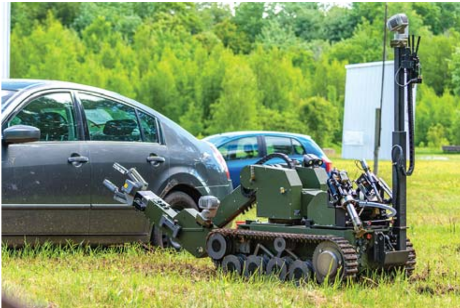
The Telerob Explosive Ordnance Disposal Observation Robot conducts a vehicle search during EOD Exercise Taz Primer.
