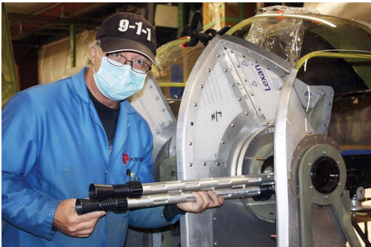
André Jean, test fitting two Browning .303 replicas to the tail turret.
