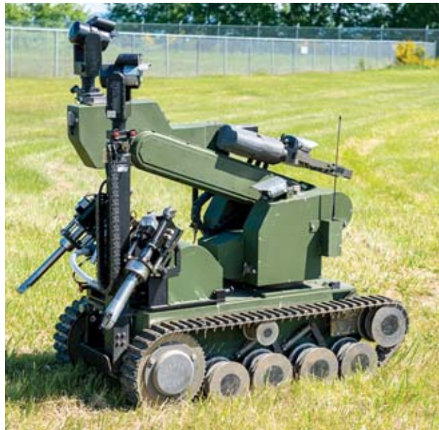
The explosive ordnance disposal robot used to disarm improvised explosive devices during Exercise TAZ RUNNER at 19 Wing Comox.
