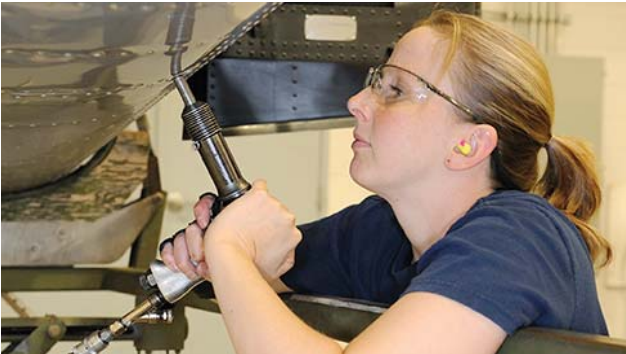
Corporal Trina Kozlik, an aircraft structures technician, rivets the exterior of the tail end of a CT114 Tutor aircraft, Cold Lake. Private K. Poudrier
