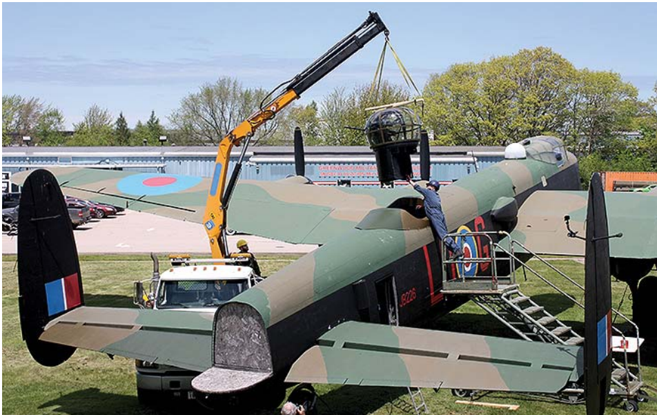
14 Wing’s Technical and Electrical and Mechanical Engineering section provided the machinery and manpower to help the Greenwood Military Aviation Museum mark a milestone in its Lancaster restoration project, placing a newly-fashioned mid-upper turret atop the display aircraft.
