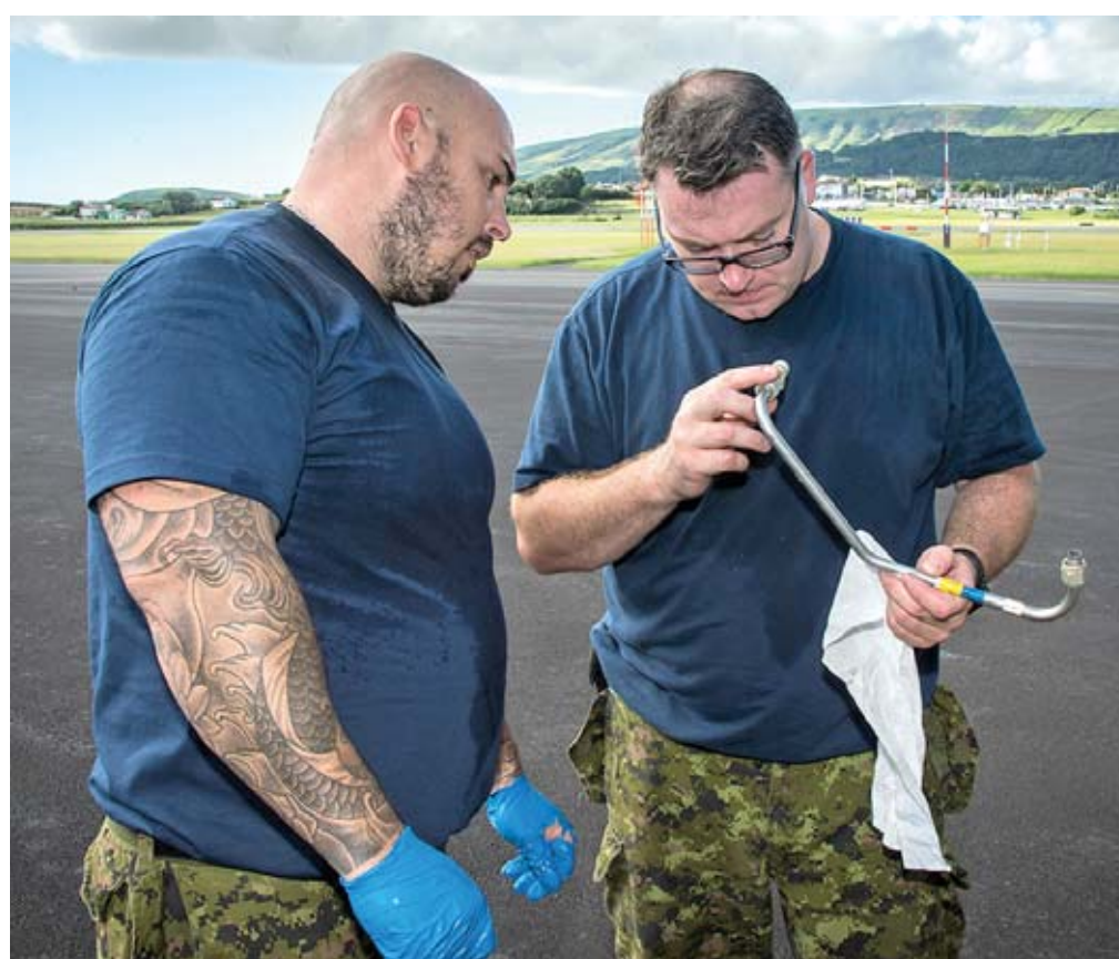
Master Corporal Mike Pittman (left) and Master Corporal Brad Dumphy, aviation technicians with 413 (Transport and Rescue) Squadron, inspect a leaking wing flap down hydraulic line on a CC130H Hercules aircraft September 21, during the Advanced Search and Rescue Exercise in Lajes, Azores.
