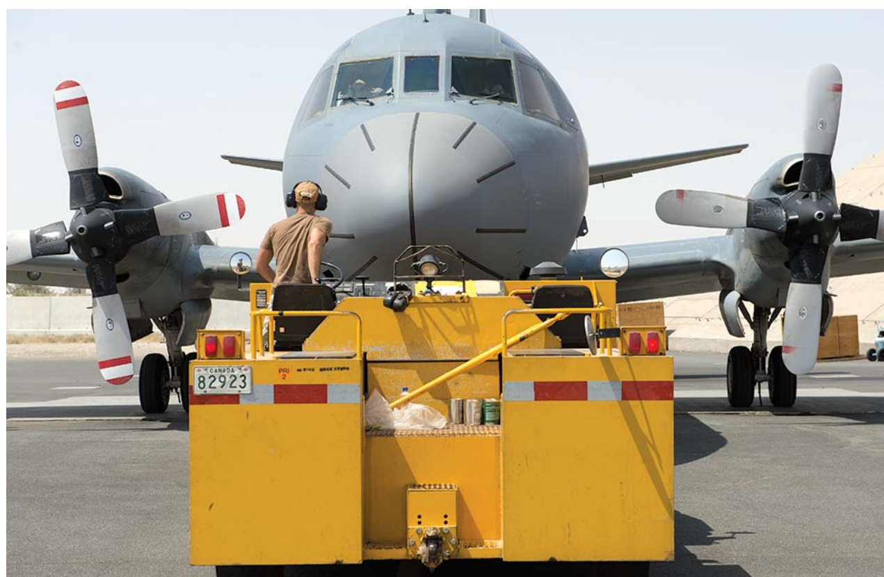
An Aviation Technician from the long range patrol detachment operates the mule to move the CP140 Aurora into position after a surveillance mission during Operation Impact in Kuwait. Operation Impact, DND
