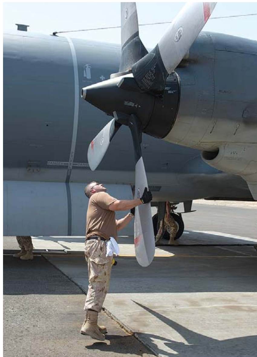
A propeller technician from the long range patrol detachment inspects the propellers for damage on the CP140 Aurora after a flying a surveillance mission during Operation Impact in Kuwait.
