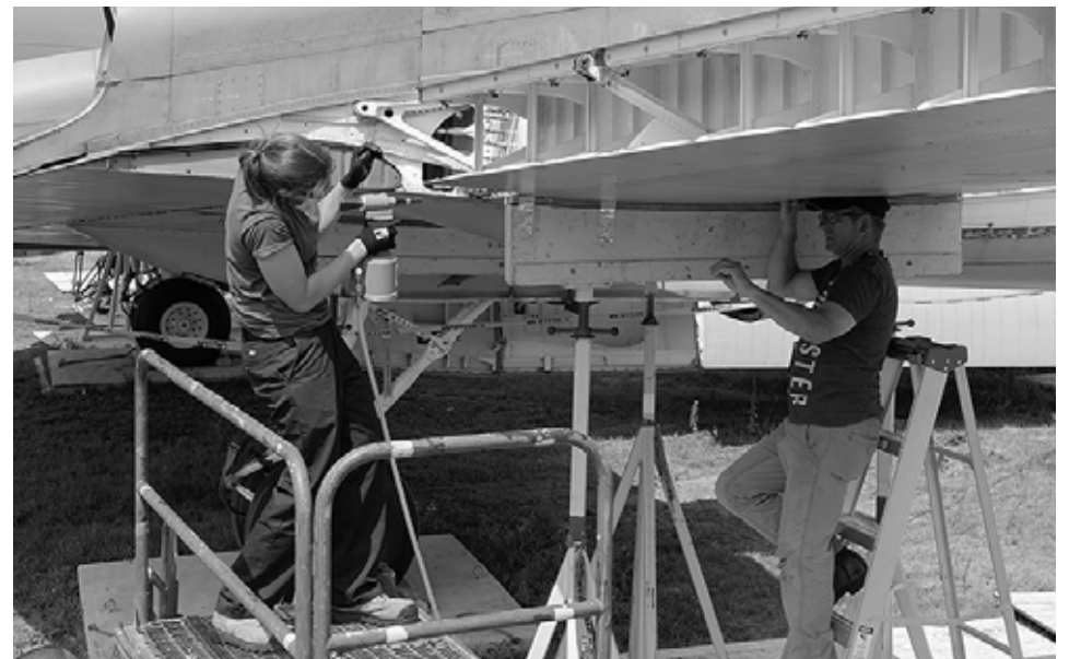
Kelsey Brown and Ira Lafort of IMP Aerospace re-attach a wing to CP140 119, at its new home in the Greenwood Military Aviation Museum's Air Park August 4.
