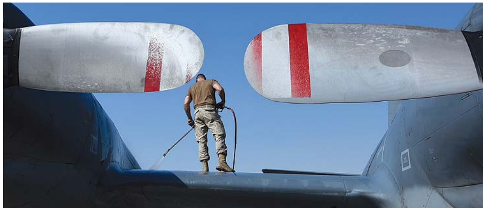
To keep the aircraft functioning properly in a desert environment, an aviation technician sprays down the wing and fuselage of a CP140 Aurora in Kuwait during Operation Impact.
