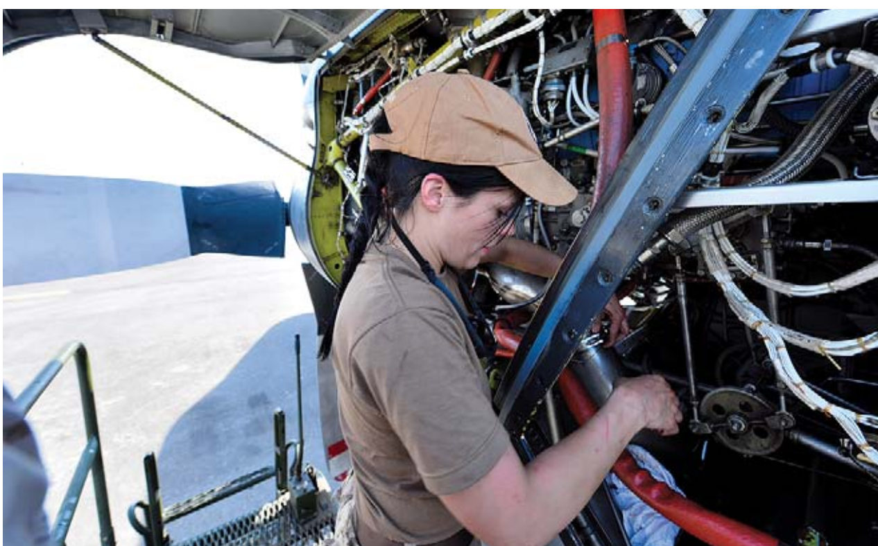
An aviation technician performs general maintenance on a CP140 Aurora engine in Kuwait during Operation Impact. Op Impact, DND
