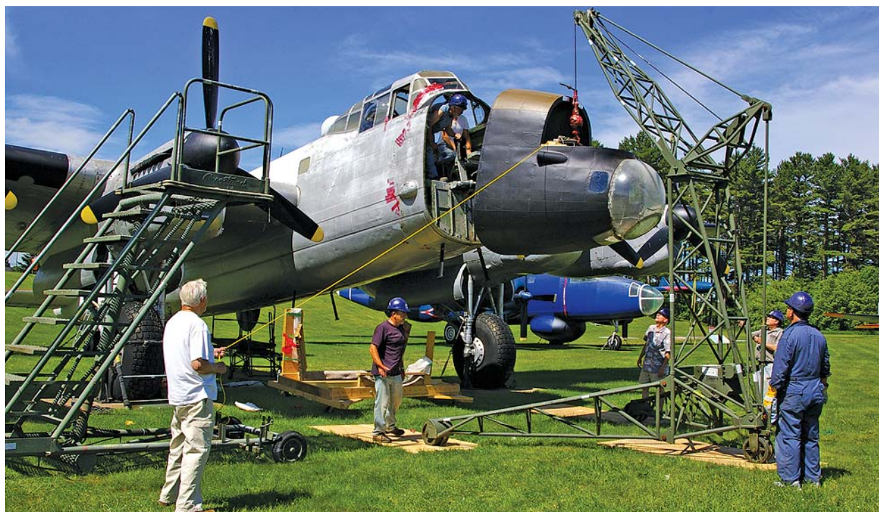
A major part of the Lancaster reconfiguration involved shortening the post-war elongated nose, refurbishing it and, here, the team is reinstalling it.
