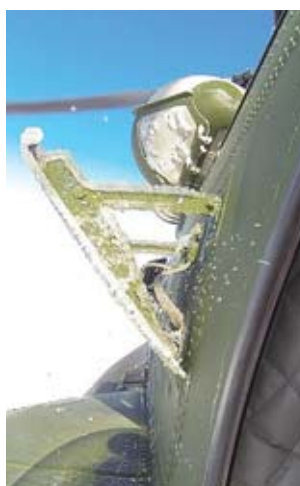
The view aft, down the right side of the Chinook during icing testing flights out of 14 Wing Greenwood through November: the picture shows the ice build-up on the airframe and engine inlet screen.
