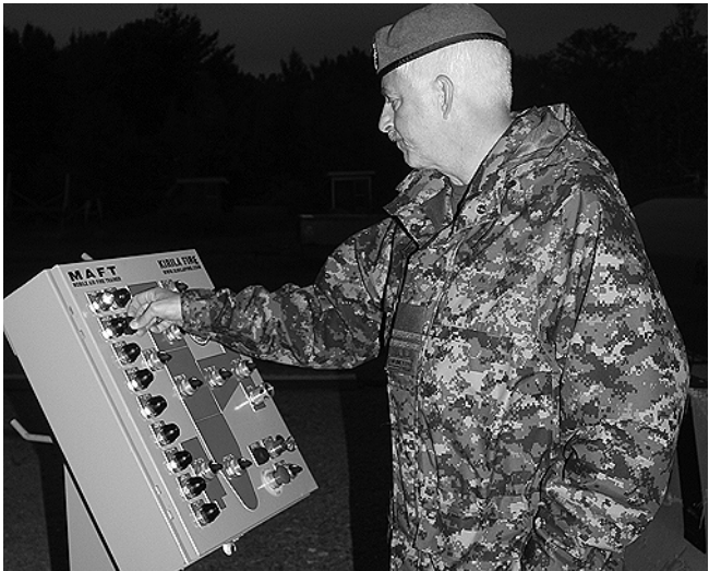
14 Wing Fire and Emergency Services Chief Captain Bruce Paradis mans the operations panel for the Mobile Aircraft Fire Trainer, and the “deadman’s switch” to activate or stop the propane fires involved in the simulated aircraft emergency trainings.
