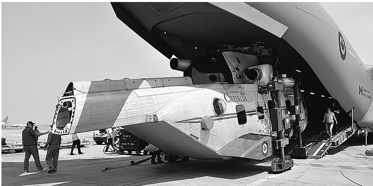
A CH149 Cormorant helicopter is unloaded from a CC177 Globemaster aircraft by IMP Aerospace technicians at the Lima airport, Peru, using the Cormorant "Air Transport Kit," a hydraulic and power assembly mounted to the helicopter itself that enables its quick and expedient loading and unloading.
