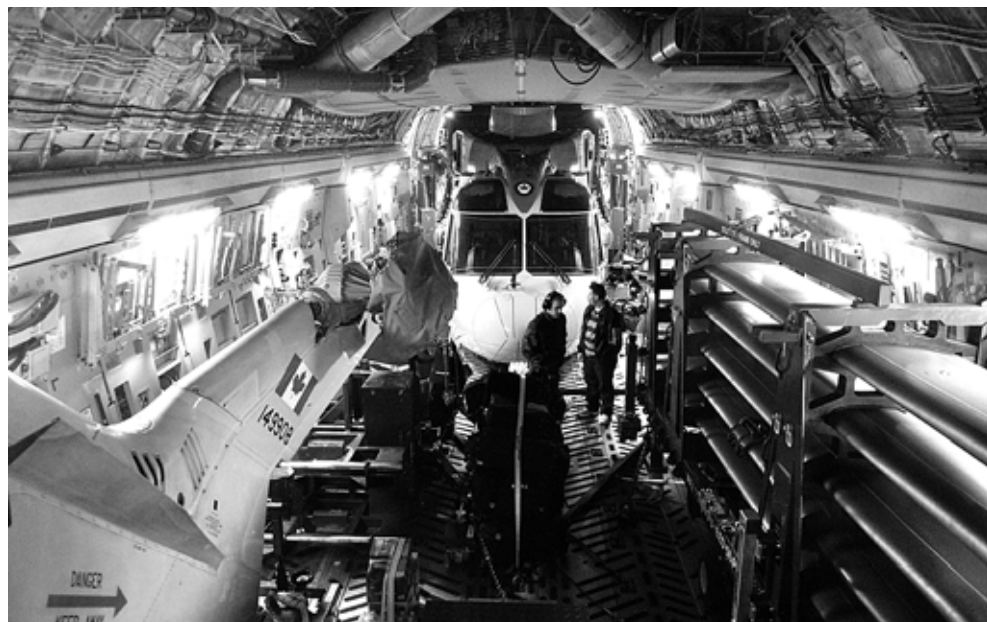
A CH149 Cormorant helicopter is unloaded from a CC177 Globemaster aircraft by IMP Aerospace technicians at the Lima airport, Peru, using the Cormorant "Air Transport Kit," a hydraulic and power assembly mounted to the helicopter itself that enables its quick and expedient loading and unloading.
