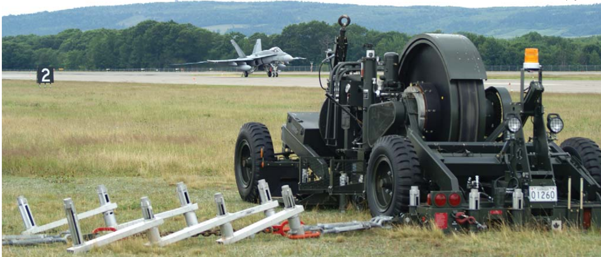
An F-18 engages the mobile arrestor cable system during installation testing on CFB Greenwood's airfield.
