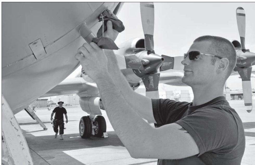
Aviation technician Private Chris Cole of Task Force Libeccio applies protective plugs and covers to sensors on a CP-140 Aurora long-range patrol aircraft. (Image: Corporal Jackson Yee)
