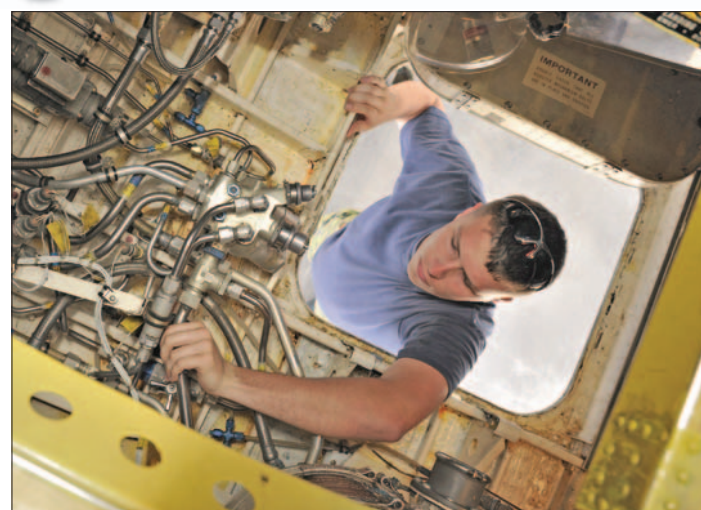
Aviation technician Cpl Alex Jalbert-Landry of Task Force Libeccio looks for leaks in the hydraulic service centre of a CP-140 Aurora long-range patrol aircraft.
