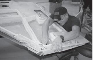
MCpl Jean Francois Tremblay (404 Sqn) works at removing foam used as a field repair to damaged (Image: D. Saulnier) wing skin.
