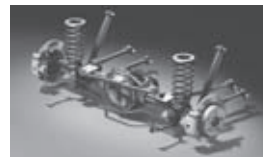
Segment exclusive* five-link coil spring rear suspension
