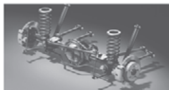
Segment exclusive▲ five-link coil spring rear suspension
